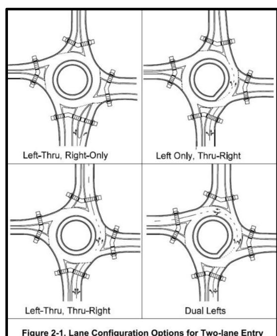
Figure 2-1. Lane Configuration Options for Two-lane Entry
