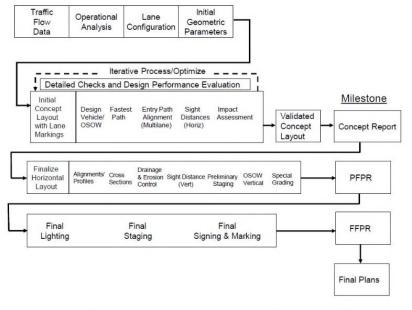
Figure 3-1. Design Process and Workflow for GDOT PDP Roundabouts
