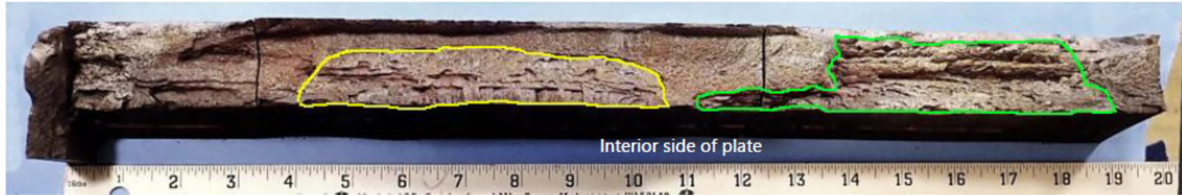
Figure 20. Lower portion of fracture showing Primary Preexisting Crack Region (yellow) and the Secondary Preexisting Crack Region (green).
