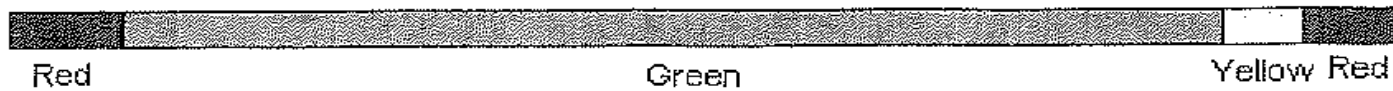
The flow of traffic during the green period from a saturated approach
